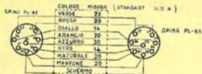
Fig. 20 - Cablaggio dei cavi CD-226, CD-239, CD-346, CD-324, CD-472, CD-676, CD-1172.
